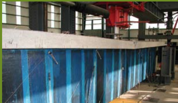
A beam strengthened with carbon fiber-reinforced polymer (CFRP) undergoes testing at the Kiewit Center for Infrastructure and Transportation at OSU.
