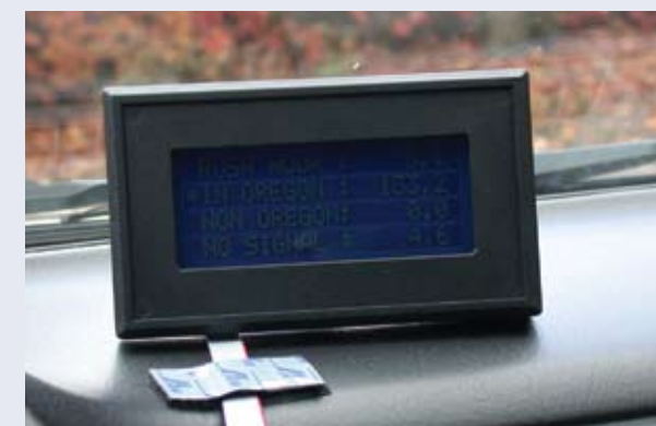
In-vehicle display that tracks mileage traveled as part of a vehicle mileage tax pilot program in Portland, OR.
